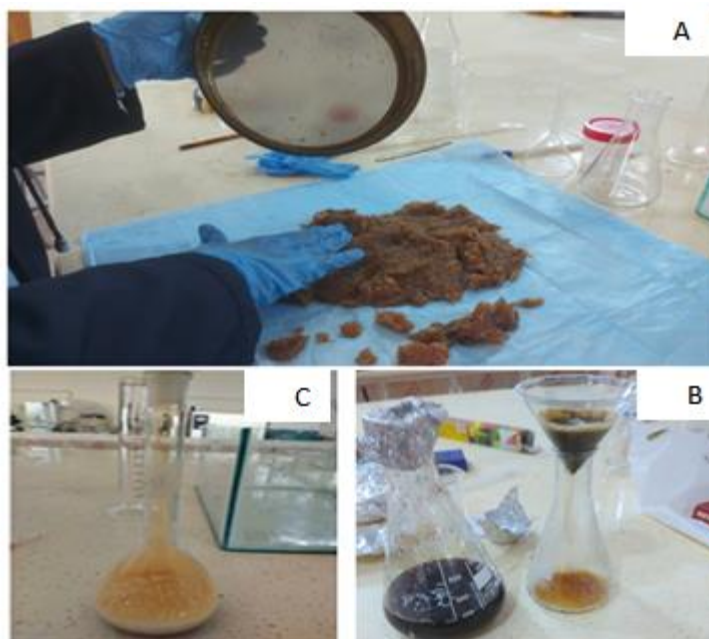
Figure 2. Steps for preparing nano chitosan in the laboratory: (A) drying shrimp, (B) chitin after adding HCl acid, (C) chitosan after adding NaOH
