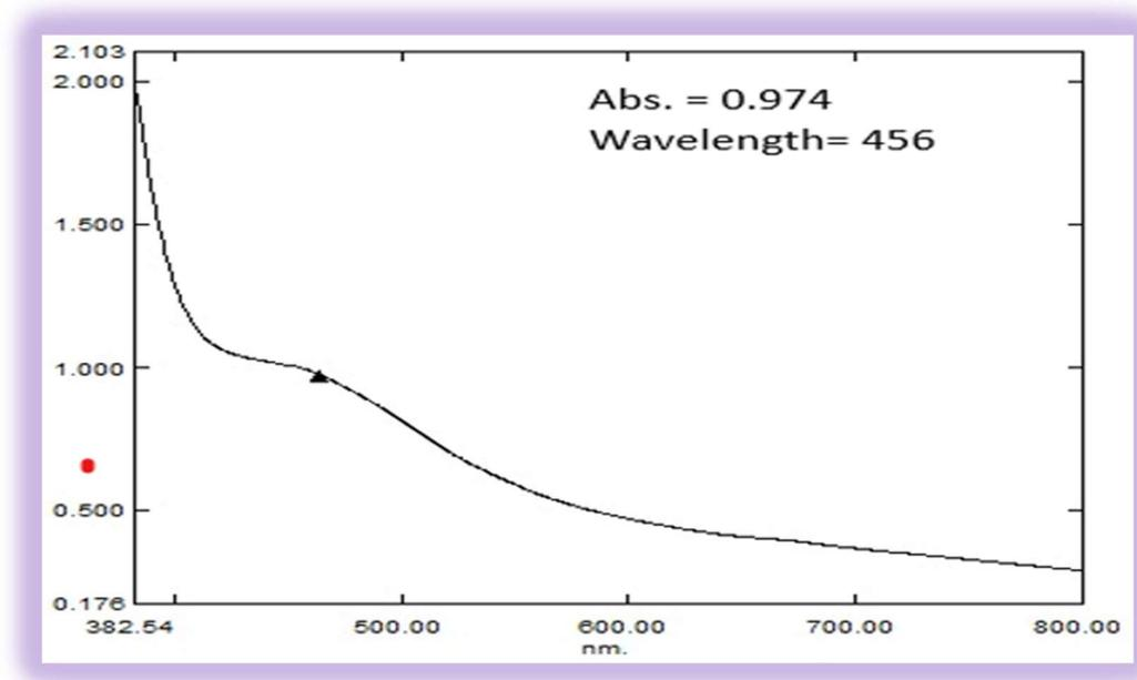
Figure 5. UV-visible Spectrophotometer spectrum examination of a sample of silver NPs prepared by using green tea *Camellia sinensis* extract
