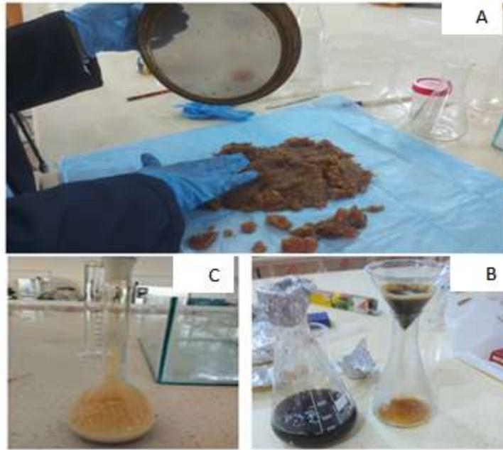
Figure 2. Steps for preparing nano chitosan in the laboratory: (A) drying shrimp, (B) chitin after adding HCl acid, (C) chitosan after adding NaO
